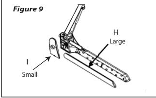
**Step #12** Snap on the left and right bracket covers (small and large covers) (see Fig. 9).
